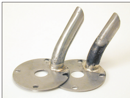
A controlled atmosphere eliminates oxidation.
